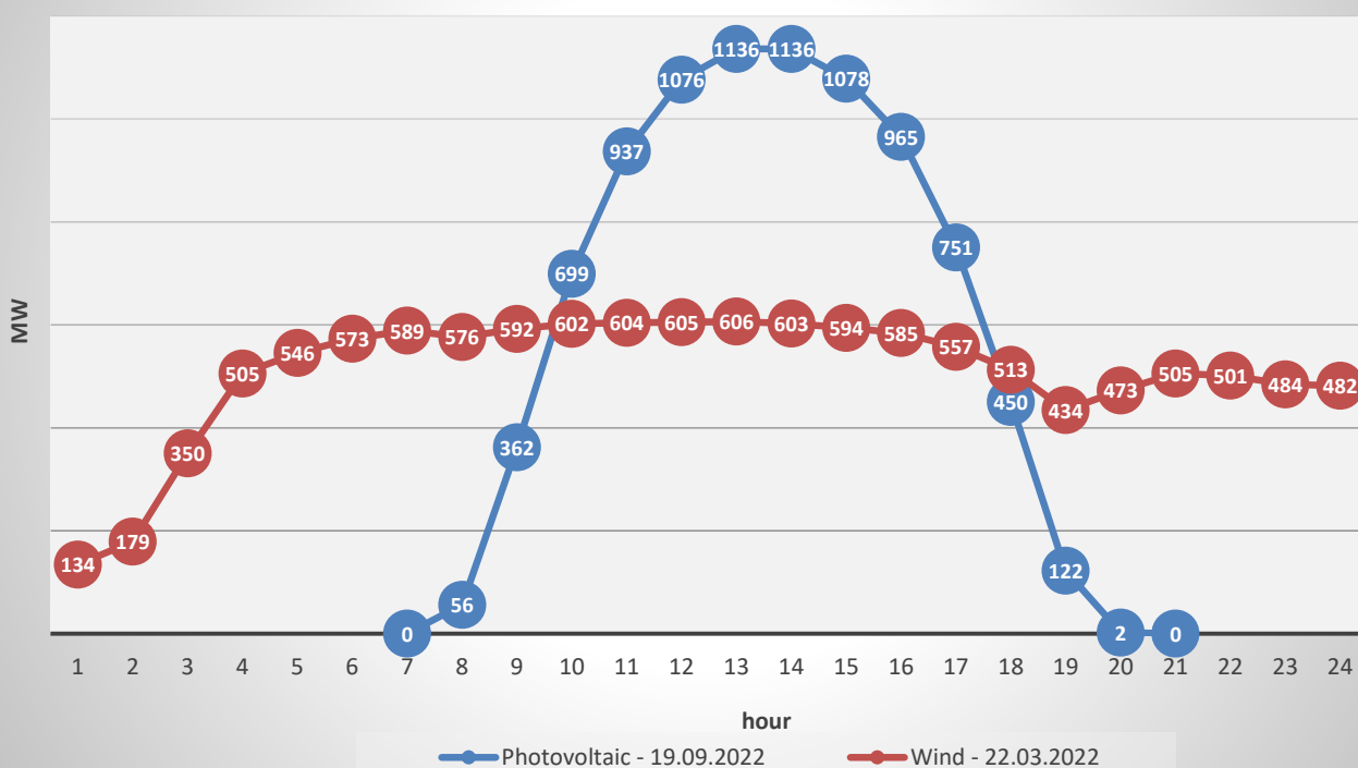
Daily generation curves of Wind and Photovoltaic for the respective days with the highest (MW) hourly generation for 2022
